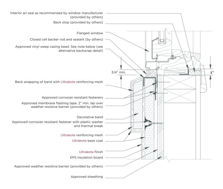
NOTE: At horizontal wall surfaces, including ledges, caps, sills, etc. a minimum slope of 6 inches in 12 inches is required.
